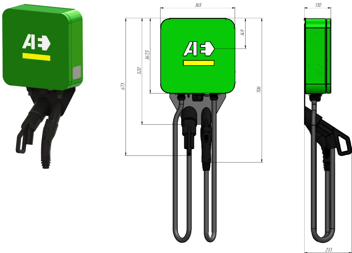
Figure 1a. Station external view and station dimensions for wall mounting (Type 1, Type 2)
